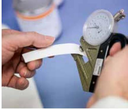
**Measurement of the layer thickness of a bare coating film in preparation for the elongation at break measurement for determining the flexibility of the coating.**
